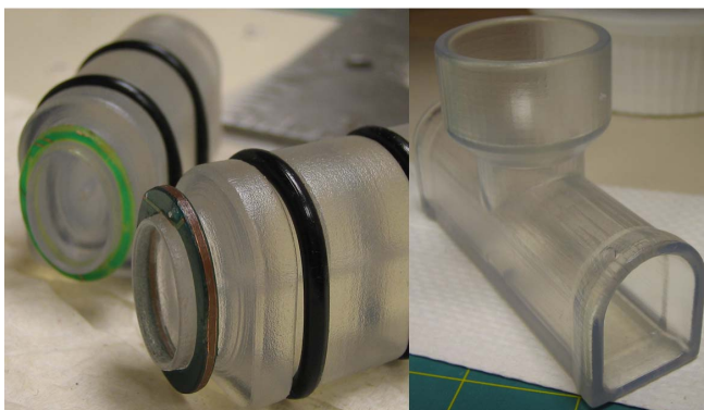
Fig. 2. Fixtures used in prototype bubble manufacturing process. Silicone film is stretched onto the plungers on the left. After some processing, the plungers are then inserted into the side cavities of the housing fixture shown on the right.
