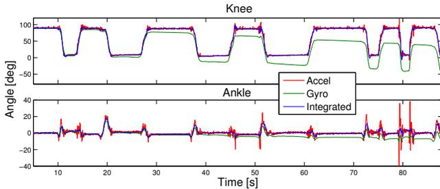
Fig. 3. Sit-to-stand estimation using gyrometers and accelerometers only.
