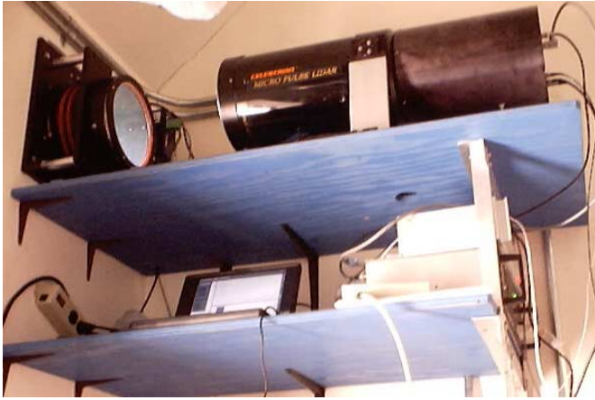
Figure 1 MPL instrument with sidewall mirror scanner installation at the South Pole atmospheric research observatory.
