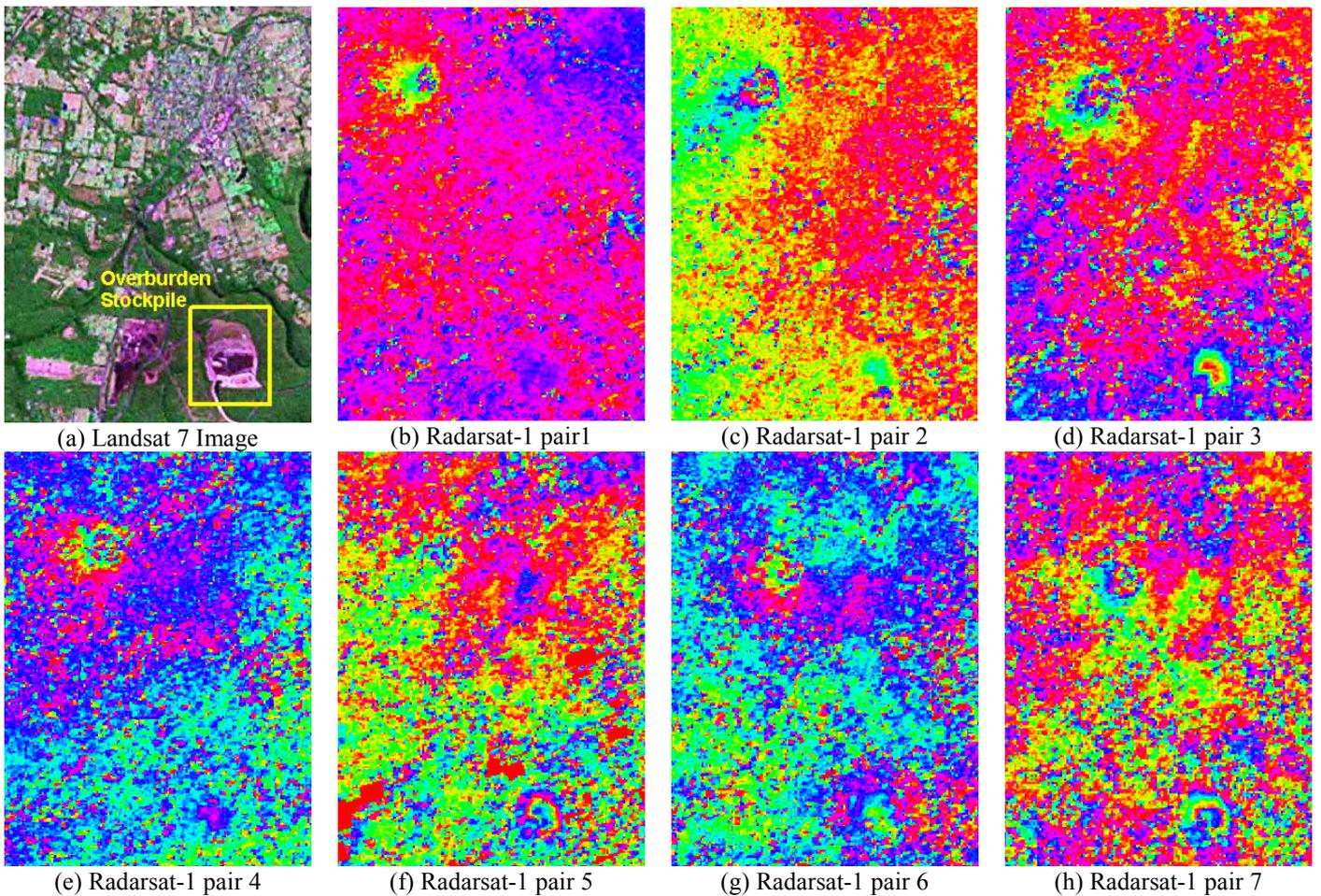
Figure 2. Landsat 7 image (a) and Radarsat-1 C-band differential interferograms derived from InSAR pairs listed in Table II with time interval of 24 days (b)~(h).
