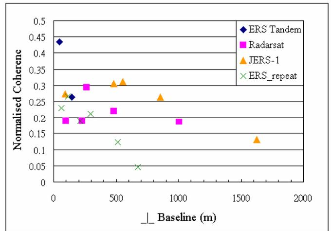
Figure 1. The normalised mean value of the coherence of the ERS-1/2, Radarsat-1 and JERS-1 InSAR results with their single repeat-pass period.
