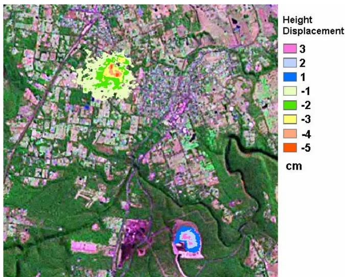
Figure 3. The colour coded DInSAR height displacement map of Radarsat-1 pair number 3. Positive height displacement indicates the increase of surface height and vice versa.
