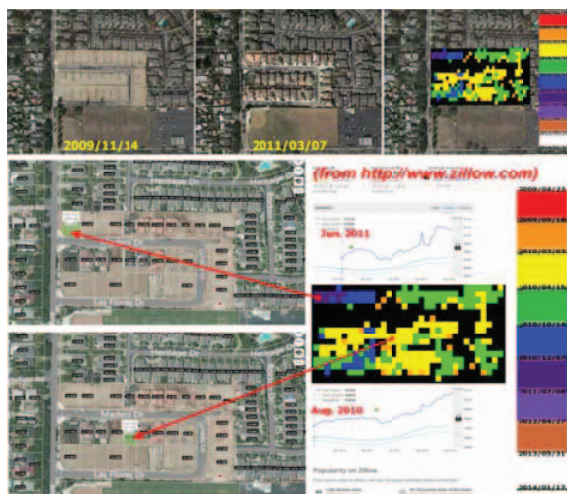
Fig. 5. Detection of building completion dates using the coefficient of Eq. 11. The comparison with the housing information provided by a real estate website (zillow.com) showed a reasonable agreement.
