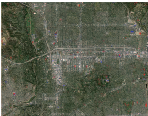
Fig. 4. Change detection results (overlaid on Google Earth image) after fitting a hyperbolic tangent function. The red and blue dots represent destroyed and constructed buildings, respectively.
