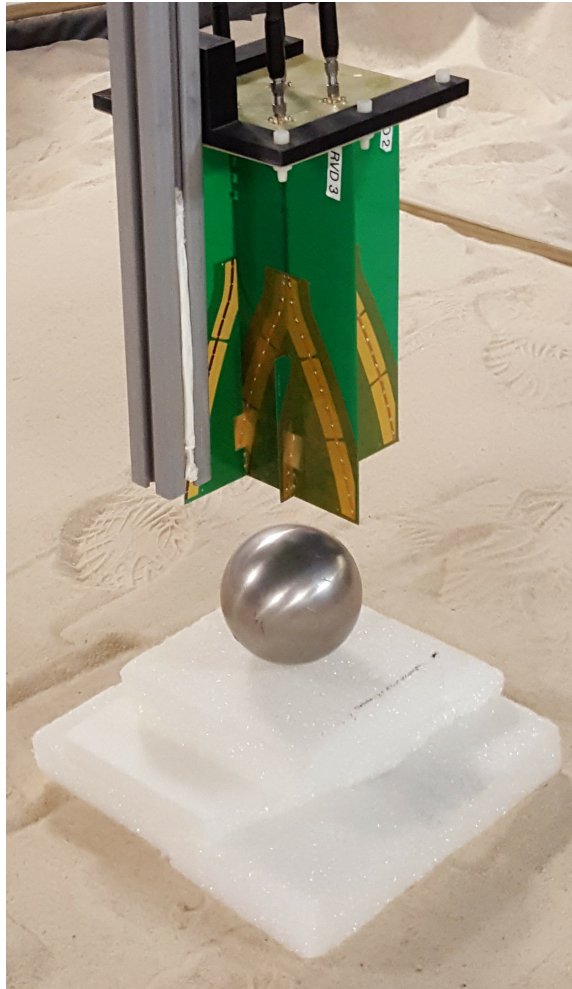
Figure A.2: Photograph of antennas with 11 cm sphere on 12 cm of styrofoam
