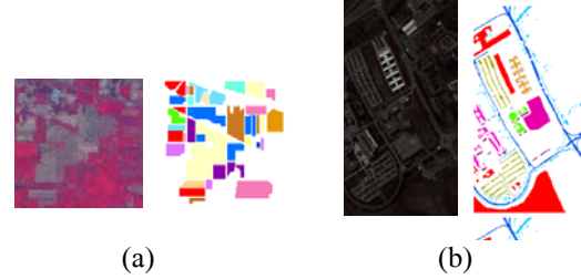
Fig. 2. The (left) false color composite image bands (bands 50, 27, 17) and (right) ground truth for two data sets: (a) Indian Pines; (b) University of Pavia.
