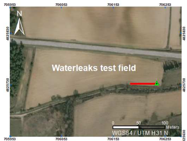
Figure 1: Waterleaks test field. The green mark corresponds to the hydrant. The red line shows the leaking pipeline.
