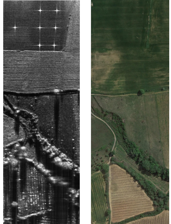
Fig. 6. SAR-Light SAR image at X-band VV polarization – incidence 75^\circ - Calibration area - Left: SAR image. Right: GoogleEarth view.
