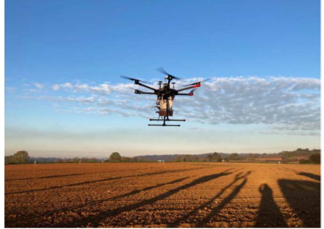
Fig. 1. SAR-Light – The new ONERA SAR sensor onboard a DJI M600 UAV.
