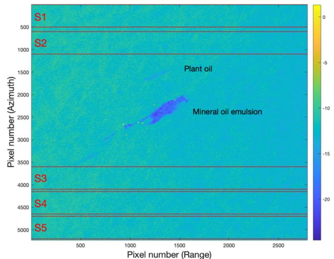
Fig. 1: Intensity image ( $\sigma_{VV}^0 [dB]$ ) of Radarsat-2 scene acquired on 11 June 2013, 17:18 UTC, multi-looked by 9x9 window.
