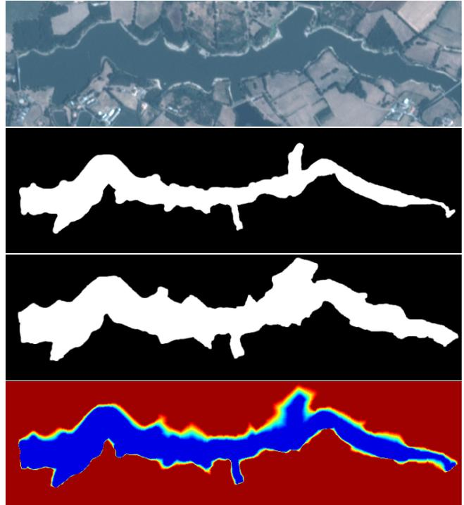
**Fig. 1.** From top to bottom: An example of a PlanetScope image of the lake of La Bultière, the mask corresponding to the empty lake surface, the mask of the surface of the filled lake, the DEM estimated using the two masks and the method presented in Section 4.
