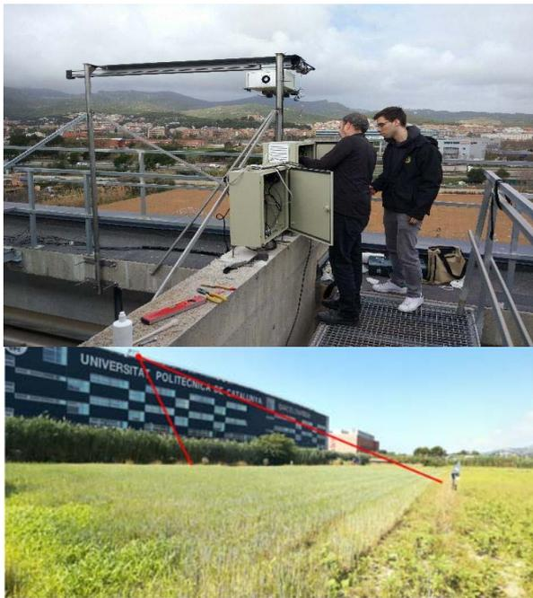
Figure 1. (Top) The Metallic structure that holds the rail is attached to the building, (Bottom) The location of the radar can be seen on the roof of EEABB building
