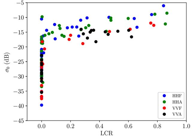
**Fig. 2.** Scatter plot of the slice  $\sigma_0$  values versus the corresponding LCR values for a set of slices in the radius of 15 km from a coastal wind vector grid cell in the Gulf of Taranto, south of Italy. Marker colours represent the different "views" of QuikSCAT. In the legend, HH (VV) stand for horizontally (vertically) polarized pulse and A (F) stands for aft (fore) beam.
