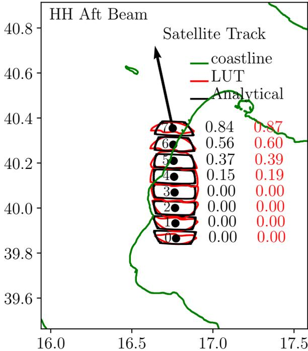
**Fig. 1.** Black (red) contours: QuikSCAT inner aft beam 3dB analytical (LUT-derived) SRF contours in the coastal area of the Gulf of Taranto, south of Italy. The slice index (0-based) is reported within each of the contours. Slice centroids are depicted with black circular markers. Black (red) text indicates the LCR values for each of the analytical (LUT-derived) contours. The black arrow depicts the flying direction of the spacecraft, while the coastline is depicted in green.
