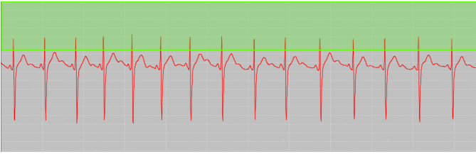
Fig. 9 Windowed filter [1] applied to a normal ECG. R-peaks are the local maxima in the filter (green shaded area at top).
