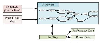
Fig. 3: The experimental setup. Preexistent files for sensor data and point-cloud map provide the real-life inputs. Profiling tools collect characterization data.
