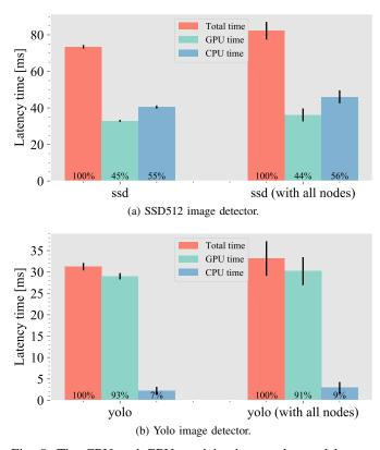
Fig. 8: The CPU and GPU participation on the total latency for SSD512 and Yolo image detectors. Two measurements were performed: vision detection nodes running standalone, and alongside all other nodes.
