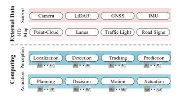
Fig. 1: A high-level description of the Autoware architecture. Sensor data and pre-existing high-definition maps feed the software stack.
