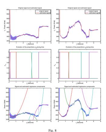
OBTAINED RESULTS FOR A SIGNAL WITHOUT DEFECT (LEFT) AND FOR A SIGNAL WITH DEFECT (RIGHT).
