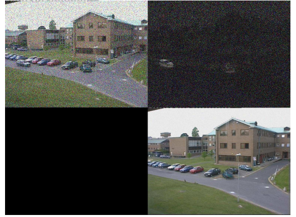
Fig. 4. The figure shows the current frame on top left, extracted foreground on top right, and the extracted background on bottom right. This is the 1003rd frame in the video sequence. Notice that the filter is phasing out the car that is leaving the parking lot from the background.
