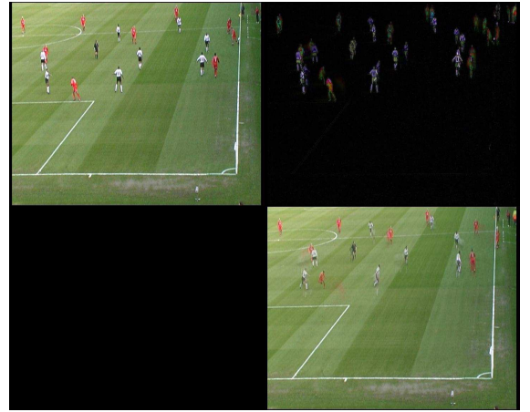
Fig. 8. The figure shows the current frame on top left, extracted foreground on top right, and the extracted background on bottom right. This is the 50th frame in the video sequence. Notice that the filter yet learning the background and there are artifacts left from the initial frame.
