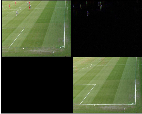
Fig. 9. The figure shows the current frame on top left, extracted foreground on top right, and the extracted background on bottom right. This is the 1283rd frame in the video sequence. Notice that the filter almost perfectly separated the foreground.
