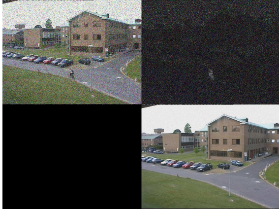
Fig. 5. The figure shows the current frame on top left, extracted foreground on top right, and the extracted background on bottom right. This is the 2808th frame in the video sequence. Notice that the filter adapted to the new scene with new parked car and completely discarded the bicycle rider.
