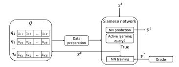
Fig. 1. Overview of the proposed method which uses a multi-sliding window approach to data storage, a siamese neural network (NN) and active learning to enable online learning from limited, nonstationary and imbalanced data.
