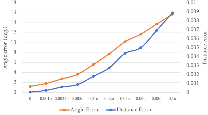
Figure 10: Angle error in degrees and distance MSE error for different levels of noise applied to the source input point cloud.
