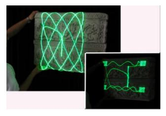
**Figure 3:** Variations of the scanning patterns, multiple Lissajous and combined Lissajous and raster/vector imaging.
