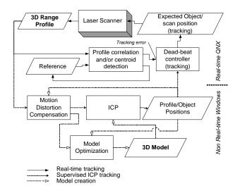
**Figure 4:** Real-time tracking consists of two feedback loops: a fast real-time linear method based on correlation and/or center-of-mass to provide stable and optimum tracking, and a non-deterministic quasi real-time supervisory loop using the proposed ICP based algorithm.
