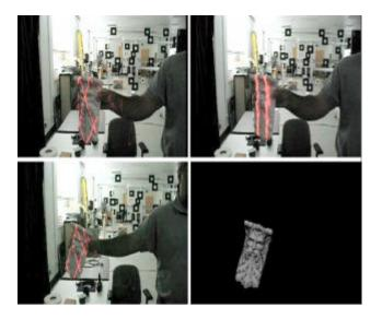
**Figure 5:** Tracking and imaging video sequence. Topleft: the system searches for an object within the field of view of the scanner; top-right: the object is found and a very low-resolution distorted model is created; bottomleft: tracking is resumed and the model refined; bottom-right: results of tracking and model creation.
