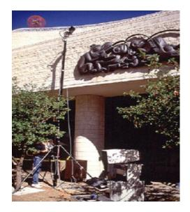
**Figure 1:** Range sensor mounted on a tripod; stability is paramount in acquiring high accuracy range images. Accuracy of range data is the combination of the range sensor and its mechanical supporting structure. Vibrations and oscillations induced by winds or passing vehicles can seriously affect accuracy.
