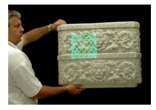
**Figure 2:** Hand-held acquisition using fast Lissajous scanning patterns and real-time tracking using the 3D range data. External constraints imposed in Figure 1 or by using external trackers are completed removed; no external equipment is needed. This is one of the experimental configurations we used during this work, the exactly equivalent opposite being holding the 3D camera.
