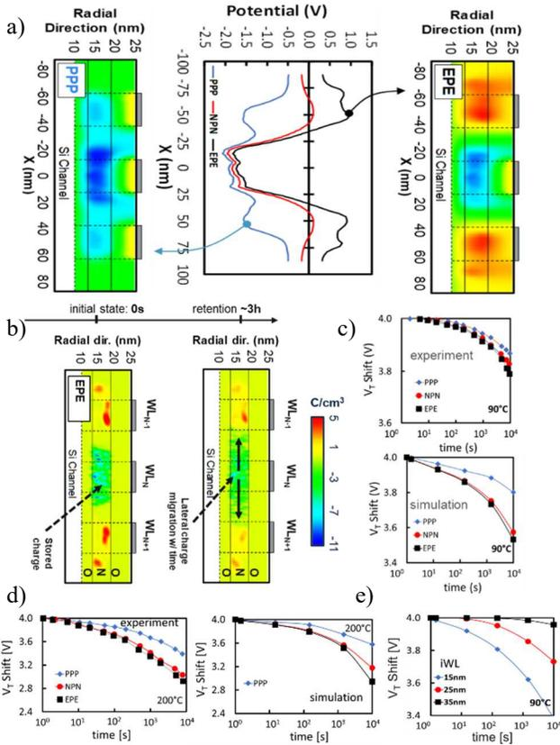
Fig. 4. a) Cell cross-section and resulting internal field generated due to the E-P-E/ P-P-P and N-P-N modes of the array. b) retention loss due to the lateral charge migration driven by the internal field. Comparison of different string modes at elevated temperatures: c) 90°C and d) 200°C. e) impact of the iWL on the P-P-P, N-P-N and E-P-E modes.
