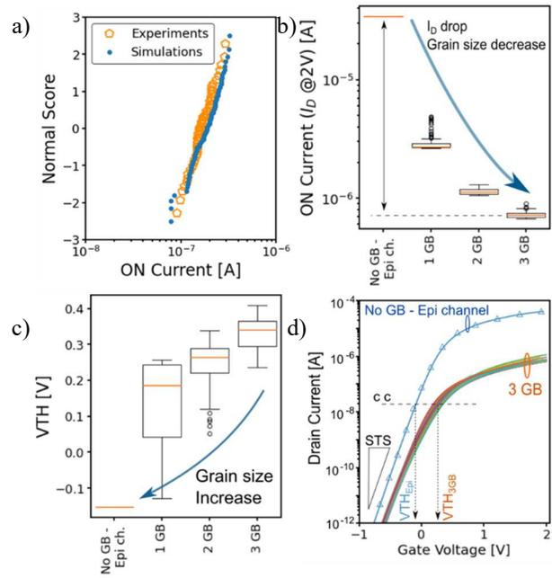
Fig. 3. Channel and taper angle induced variability. a) Calibrated ON current at overdrive voltage. b) ON current reduction and c)  $V_{TH}$  decrease with grain size decrease. d) 100x ON current increase with transition from polySi to epitaxial channel.
