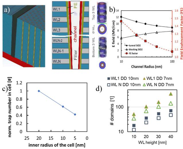
Fig. 2. 3D NAND stack with focus on a) taper angle and b) diameter change induced voltage divider modification across the stack along the string. A number of c) defects and a number of d) domains inside the storage part of the cell depending on the: 1) inner radius of the cell, 2) WL width and domain diameter - DD.
