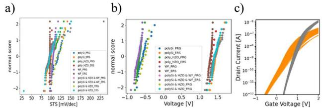
Fig. 6. Variability of the 3D FE NAND. a) STS and b)  $V_{TH}$  of PRG and ERS deconvoluted based on the variability source. c) Comparison of the CT and FE based cell (orange – CT and gray – FE device).
