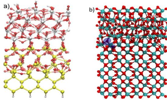
Fig. 5. Structures used in DFT simulations. a) The Si/SiO<sub>2</sub>/HZO stack used to calculate properties of defects at SiO<sub>2</sub>/HZO interfaces. b) The (o)-HfO<sub>2</sub>/amorphous (a)-HfO<sub>2</sub> interface used to study electron trapping at GBs.
