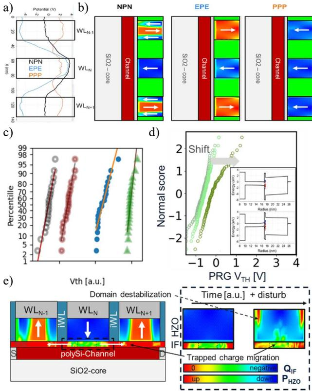
Fig. 7. a) Field distribution across the 3 adjacent WLs and their b) polarization configuration Retention. c) MLC capability of the cell and d) retention loss of PRG state due to the disturb ( $V_{\text{pass}}$ ) and e) lateral charge migration inside the  $\text{SiO}_2$ . Inset inside d) denotes causality of flipped domain and compensating charge at interface observed on band diagram.
