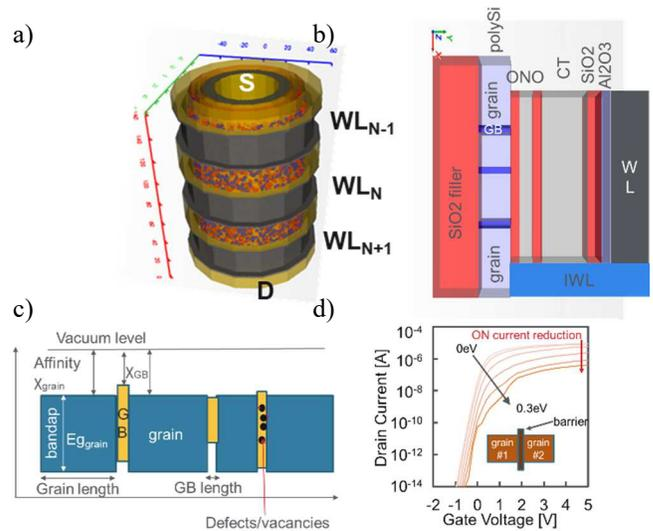
Fig. 1. a) 3D NAND string; b) cross-section of the CT 3D NAND device with depicted grains and grain-boundaries within the channel; c) Channel with grains and GBs in the energy domain. d) ON current degradation and  $V_{TH}$  hike toward higher  $V_G$ -s with increasing GB barrier.
