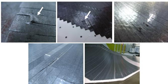
Figure 1: Various kinds of defects, such as wrinkles, early cut tapes, foreign objects (top row), and large gaps (bottom row).
