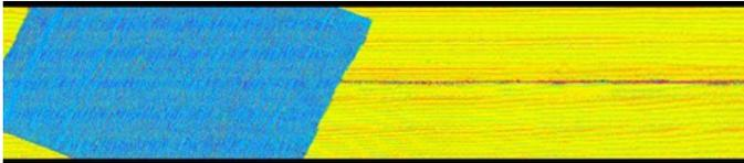
Figure 4: Fiber orientations from 5 sensors merged together to a single color-coded fiber orientation image. The blue area shows a patch of material with different fiber orientation and the dark line indicates a gap.
