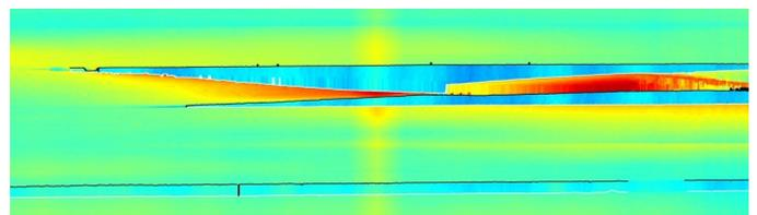
Figure 3: Depth image of a "twisted tow" defect and gap defect recorded by a laser profile scanner. Red color indicates elevated regions, blue indicates low regions.
