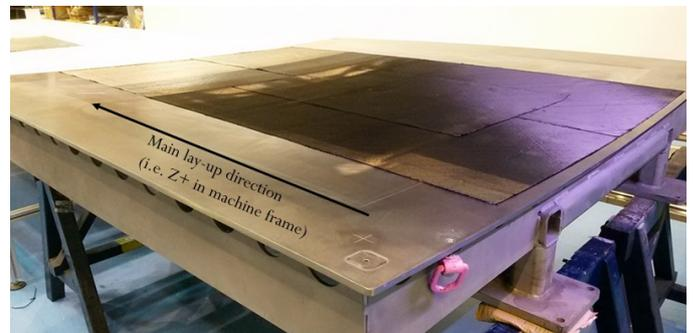
Figure 8: Setup for ADMP part manufacturing. Carbon fiber material is automatically placed and inspected.
