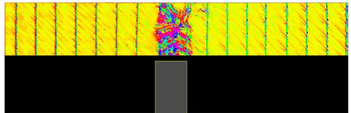
Figure 2: Detail in fibre orientations: color-coded fiber orientations (top) with defective region of unstructured material and the corresponding detection result indicated as a bounding box (bottom).
