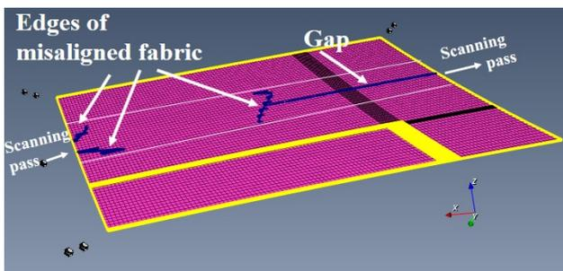
Figure 9: Features representing ply boundaries and gap back-projected onto the surface of manufactured part.
