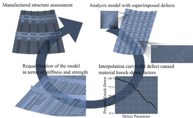
Figure 7: Analysis method to efficiently determine the effects of defects in a composite part [1].
