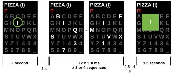
Fig. 1: Protocol design using P300-speller paradigm for recording positive or negative feedback-related responses [16].
