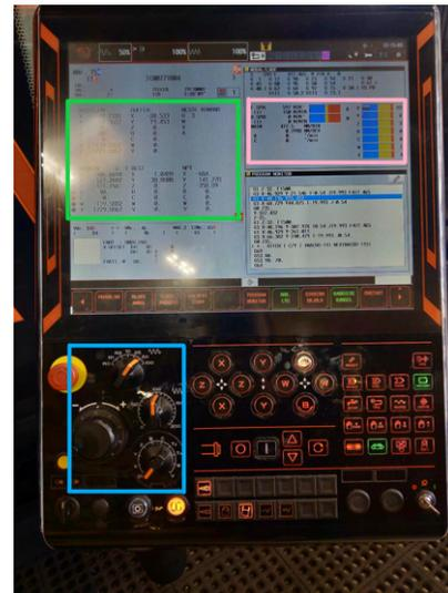
Fig. 2. Mazak Integrex i500 control interface. The green box shows information about the cutter's positions. The pink box shows information about different loads on the cutter. Inside the blue box are the knobs for controlling engagement rates.
