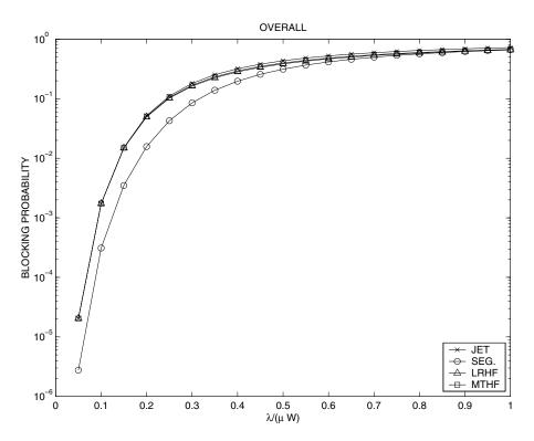
Fig. 5. Overall blocking probabilities using JET, Seg., LRHF and MTHF policies
