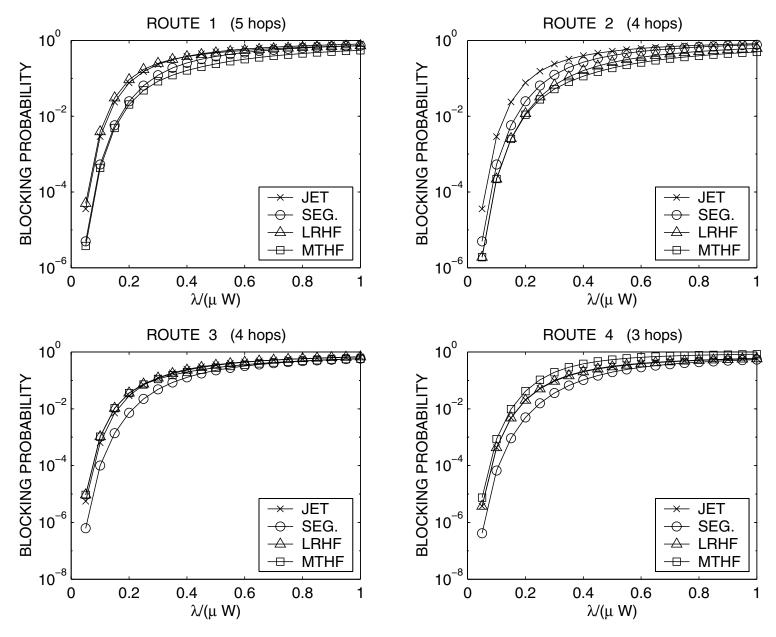
Fig. 2. Route blocking probabilities using JET, Seg., LRHF and MTHF policies
