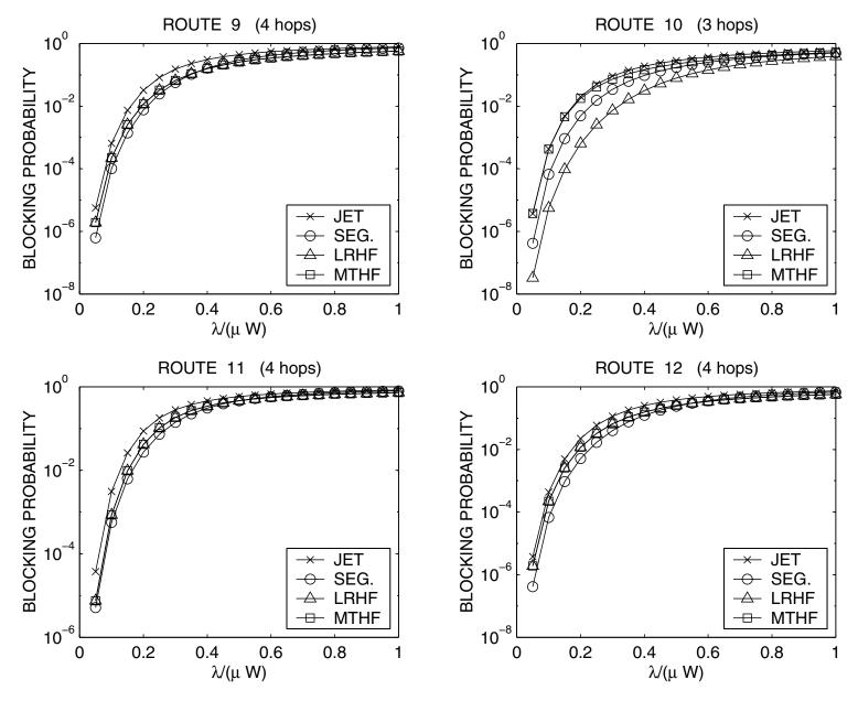
Fig. 4. Route blocking probabilities using JET, Seg., LRHF and MTHF policies
