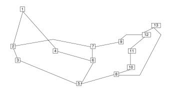
Fig. 1. NSFNET backbone network (T3, 45 Mb/s, April 1995).
