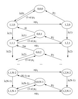
Fig. 6. State transition rate diagram of node  $i, i = 1, \dots, P$ , of the queueing network of Figure 5
