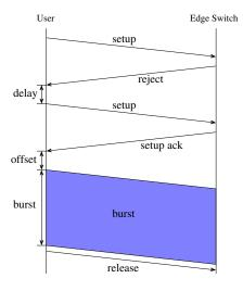
Fig. 1. Signaling messages in JumpStart
