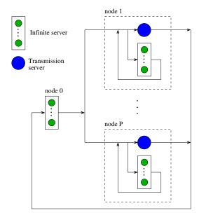
Fig. 5. Queueing network model of a sub-system of an edge switch without converters
