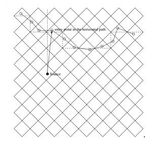
Fig. 5. A source transmits packets directly to the entry point on a horizontal path.
