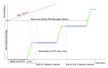
Fig. 1. The GTS (b,r)-based performance model.
