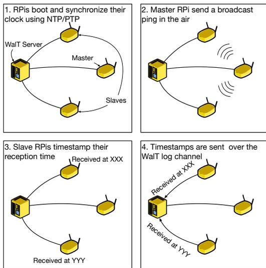
Figure 4. Clock drift measurement scenario
