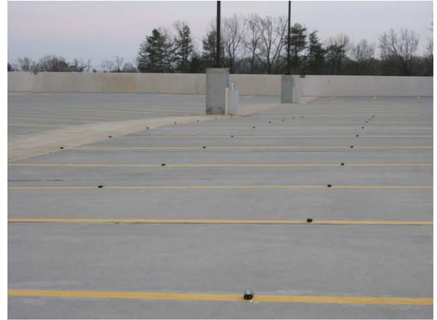
Fig. 4. Outdoor 3x11 TelosB testbed
