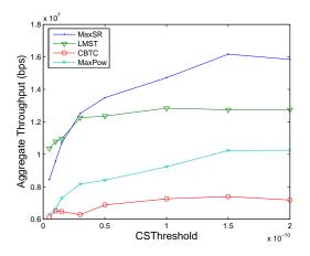
Fig. 7. Aggregate throughput v.s. carrier sense threshold
