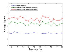
Fig. 2. Average interference degree v.s. average node degree
