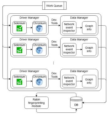
Fig. 5. ORM high-level structure diagram
