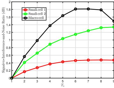
Fig. 7. SINR versus different values of  $T_a$ .
