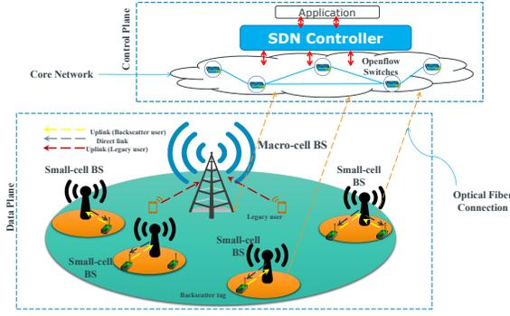
Fig. 2. Illustration of SDN-based backscatter heterogenous network consisting of macro-cell and multiple small-cells.
