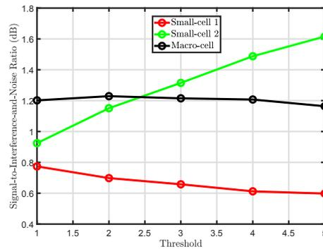
Fig. 6. Illustration of SINR for increasing values of threshold.
