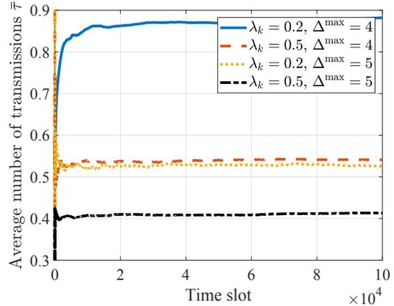
Figure 2. The evolution of the average number of transmissions,  $\bar{\tau}$ , versus time slots for different packet arrival rate  $\lambda_k$  for  $k \in \mathcal{I}$ .
