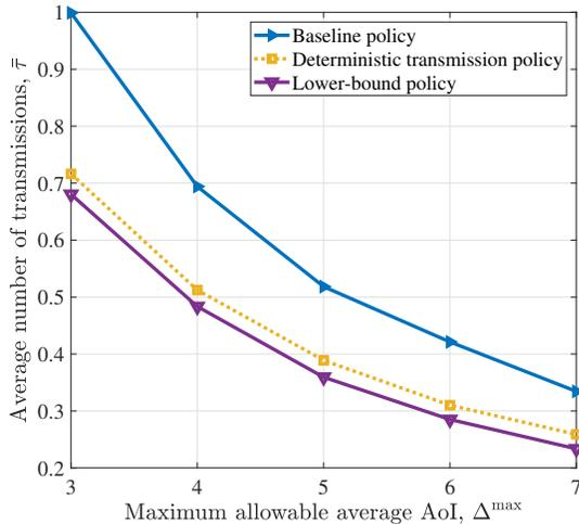
Figure 3. The average number of transmissions,  $\bar{\tau}$ , for the proposed transmission policy versus  $\Delta^{\max}$  where  $\lambda_k = 0.7$  for all  $k \in \mathcal{I}$ .
