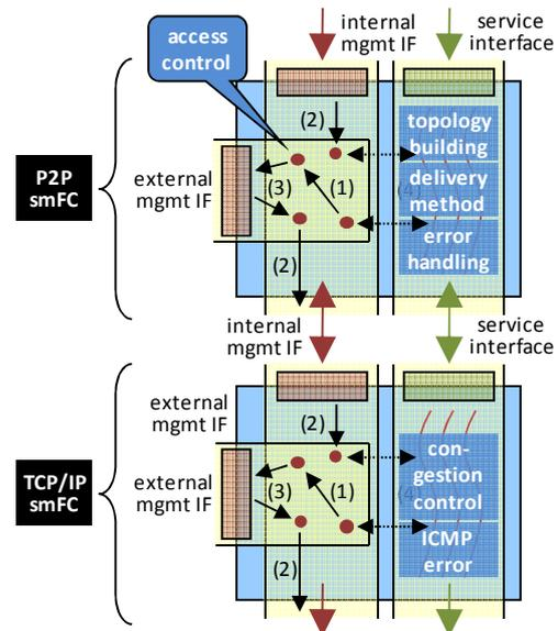
Fig. 7. Example: in-network management for P2P systems.
