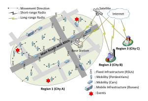
Fig. 1. Heterogeneous Architecture for Smart City Networks.
