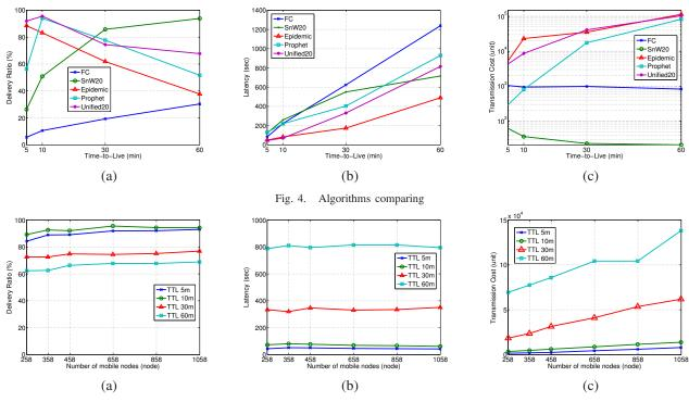
Fig. 5. Unified performance with varying the number of mobile nodes
