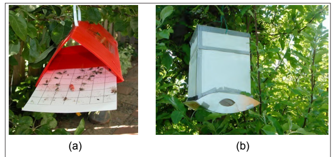
FIGURE 1. Codling moth traps: a) commercial trap; b) prototype of the IoT neural network codling moth smart trap.
