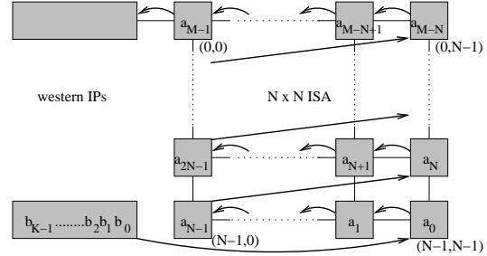
**Figure 5. Data flow for aligning two sequences  $A$  and  $B$  on an  $M = N \times N$  ISA:  $A$  is loaded into the ISA one character per PE and  $B$  is completely shifted through the array in  $M + K - 1$  steps. Each character  $b_j$  is input from the lower western IP and results are written into the upper western IP.**
