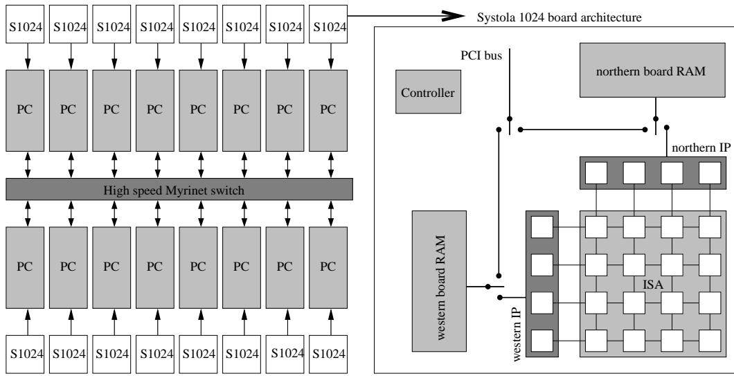
**Figure 3. Architecture of our hybrid system: A cluster of 16 PCs with 16 Systola 1024 PCI boards (left). The data paths in Systola 1024 are depicted on the right.**
