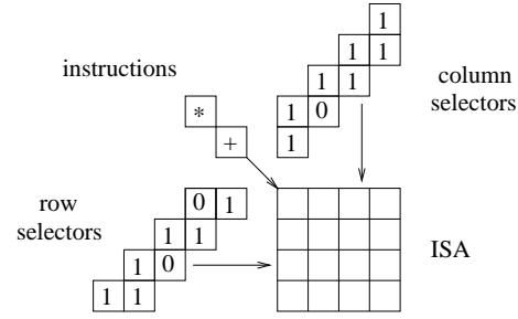
**Figure 4. Control flow in an ISA.**
