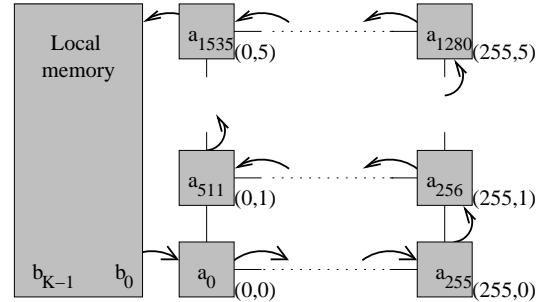
**Figure 7. Data flow for aligning two sequences  $A$  and  $B$  on the Fuzion 150:  $A$  is loaded into the processor array one character per PE and  $B$  is completely shifted through the array in  $M + K - 1$  steps.**
