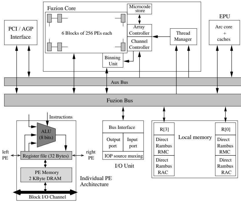
**Figure 6. System block diagram of the Fuzion 150 architecture and the architecture of an individual PE.**
