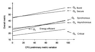
Figure 3. The effect of CPU's variation on the overall metric (average PDA)
