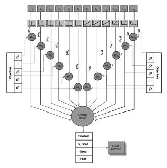
Figure 2: The calculation of the overall routing metric.
