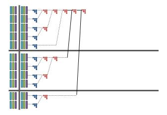
Fig. 2. Illustration of the TSQR panel factorization routine on a M-by-3 matrix. It involves only one reduction tree. Moreover the reduction tree is tuned for the grid architecture. We only have two inter-cluster messages. This number (two) is independent of the number of columns. This number is obviously optimal. One can not expect less than two intercluster communications when data is spread on the three clusters.
