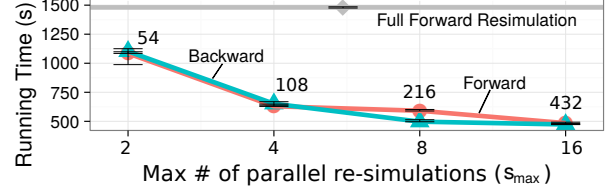
Fig. 18: Strong scalability of analyses accessing virtualized FLASH data. The data points are annotated with the number of used compute nodes.
