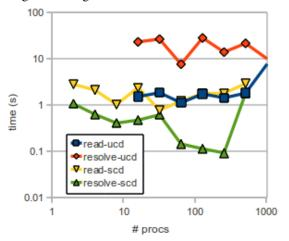
Figure 3. Execution time for parallel read and shared vertex resolution for sturctured mesh, using unstructured (ucd) and structured (scd) algorithms.
