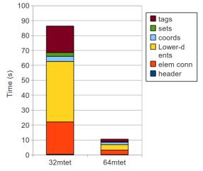
Figure 2. Distribution of read times, with (32m tet) and without (64m tet) geometry sets.
