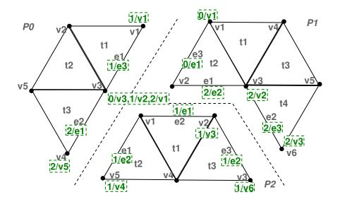
Figure 9. After shared interface resolution, with shared vertices/edges marked. Most shared entities are shared with only 1 other processor, and are marked only with the remote processor/handle. Vertex v3 on P0 is shared by all processors, and therefore local handle/processor appears in its sharing list.
