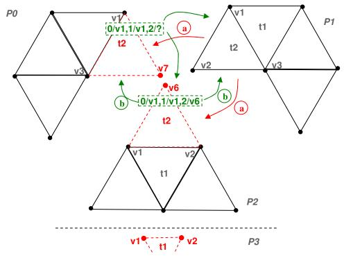
Figure 10. Ghost exchange, showing specific information for triangle t2 and its support. a) P1 sends quad t2 and vertex v1, along with sharing information 0/v1, 1/v1, 2/? for v1, to P0 and P2. b) P2 sending remote handles for v6 to P0 and P1. When P0 receives remote handles for v1, it replaces 2/? in sharing list with 2/v6 from message.
