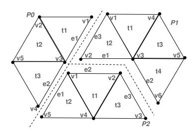
Figure 7. Mesh after initial partitioned read.
