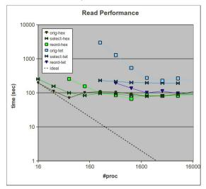
Figure 1. Read performance for 32M hex and 64M tet meshes. Original (no optimizations), select (improved selection mechanism), reord (after reordering).
