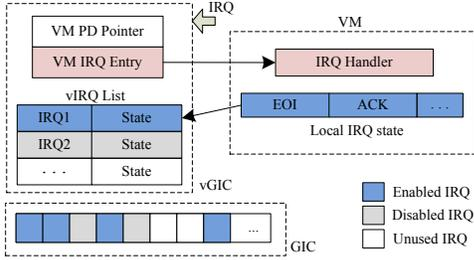
Figure 2. Structure of Virtual Generic Interrupt Controller
