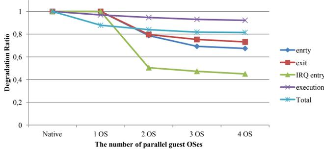
Figure 9. Performance degradation ratio of Hardware Task Manager
