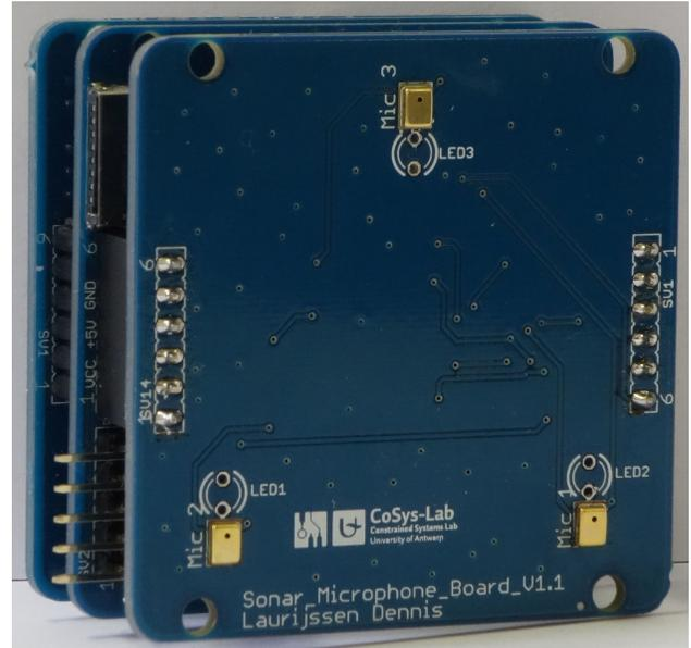
Fig. 7. Picture of a stack of three boards consisting of the core hardware board, the front add-on board with three microphones and a back add-on board which has been only been fitted with the charging circuitry and a coin cell holder. The stack measures 5cm by 5cm by 3,25cm).
