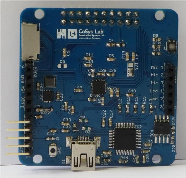
Fig. 6. Picture of the developed core hardware board (5cm by 5cm) with the (stackable) headers.
