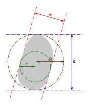
Fig. 1. Geometrical functionals of a compact set: radii of inscribed (r) and circumscribed (R) circles, minimum ( $\omega$ ) and maximum (d) Feret diameters.
