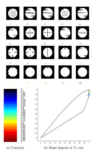
Fig. 6. Family  $\mathcal{F}_5$  of twenty 2D compact sets, represented in white on binary images. All these sets have a 'disk' shape. The color of the number is related to the convexity parameter value (a). Discrimination of similar sets for this family  $\mathcal{F}_5$  (b) mapped onto the shape diagram  $\mathcal{D}_8$ .
