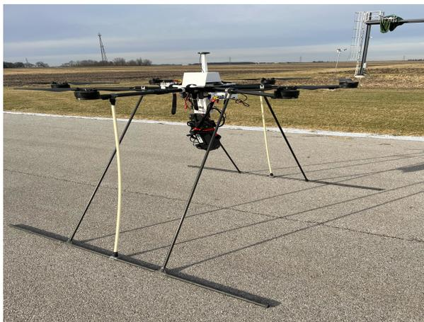
**Figure 3.3.** Self-build PhenoBee
