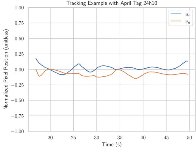
Fig. 3: Normalized pixel positions of the landing pad during an example landing. The drone is able to track the marker (i.e.  $(u_n, v_n) \approx (0, 0)$ ) by aiming the camera as it approaches.
