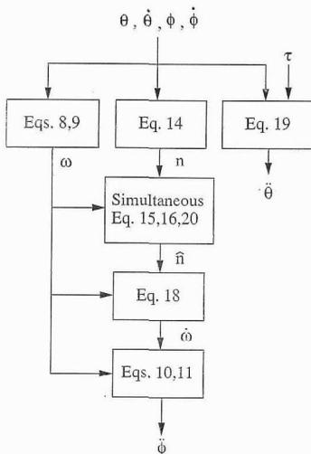
Fig. 5 Algorithm to solve direct dynamics problem of flexible arm using proposed model
