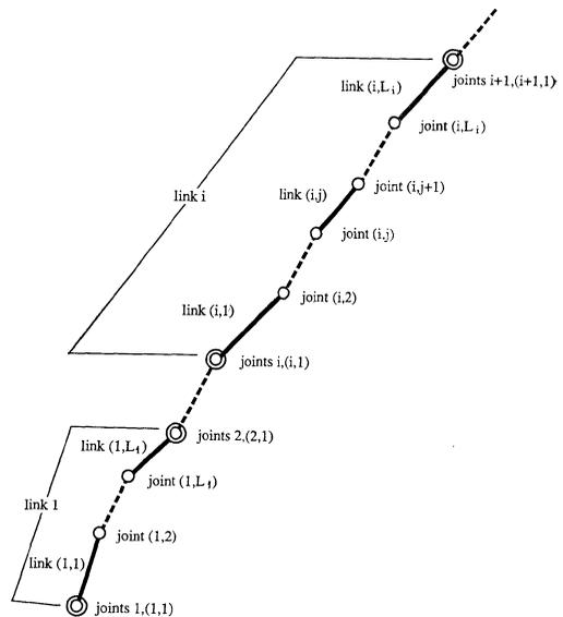
Fig. 2 Virtual links and passive joints
