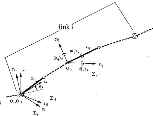
Fig. 3 Coordinate frames of virtual links
