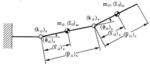
Fig. 4 Flexible link model with 1-end clamped, 1-end free
