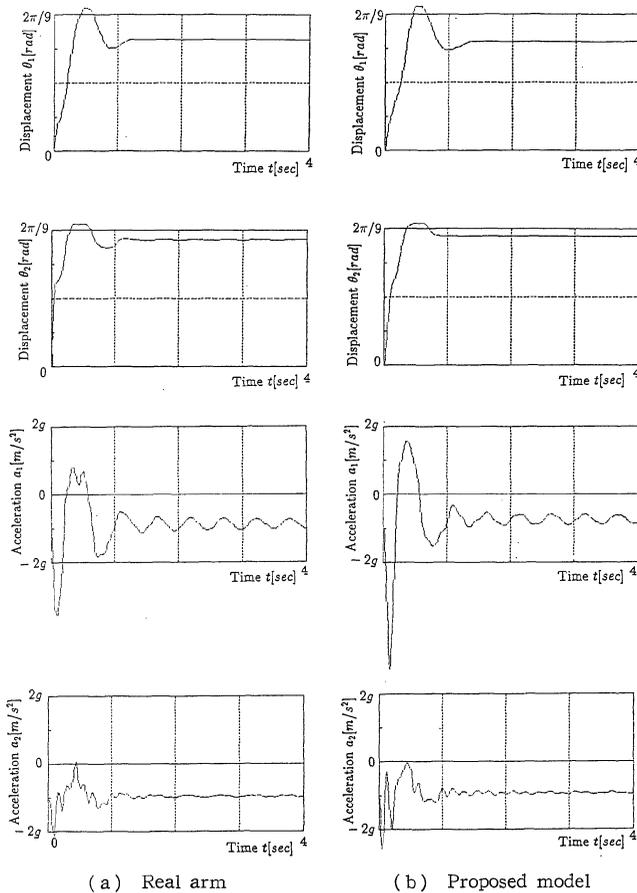
Fig. 7 Response of displacement and vibration of real arm and proposed model (the case when the joints are controlled by PD feedback)
