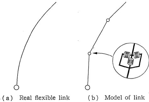
Fig. 1 Modeling of flexible link using virtual rigid links and passive joints
