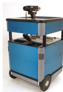
**Figure 1:** The autonomous robot Pygmalion. Its controller consists of a VME standard backplane with a Motorola PowerPC 604 microprocessor, clocked at 300 Mhz. Among its array of peripheral devices, the most important are the wheel encoders, a 360° laser range finder and a grey-level CCD camera.
