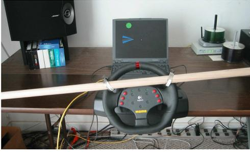
Fig. 1. Aiming device; one subject stood on either side of the wheel
